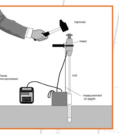
The PANDA is a light-weight (total weight of equipment 20kg) dynamic cone penetrometer, which uses variable energy and can be operated by one man to test soils in almost any location to a depth of 6 meters. The device is used by penetrating material and measuring ground or material resistance which can be conveyed in results applicable to client requirements such as MPa, KN, psi, CBR, etc.
